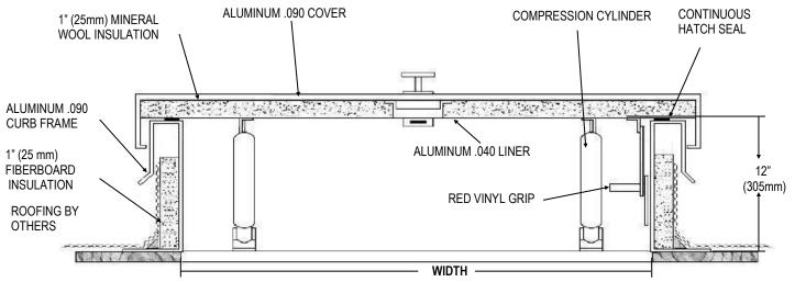
The Model RHA Series roof hatches provide for normal ladder, step ladder and stair access to roof from interior of the building. Manufactured from aluminum with weather resistant gasketing, these units feature long life, low maintenance and ease of operation. J.L. offers fully welded, mitered corners and box type door design. Units install easily over roof opening and are secured from base flange to roof deck.
