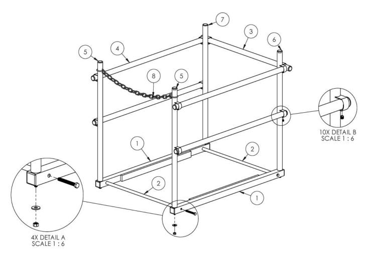
**General:** Safety railings are designed to mount on roof hatches to provide fall protection around the hatch when open. The following instructions are recommended general guidelines for installing compression type safety railings.
