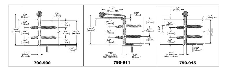
HAGER Models 790-900, 790-911, and 790-915 are Stainless Steel Continuous Edge Mount Hinges for 1-3/4" (44.5mm) thick doors. Clearance required between the hinge edge of the door and the frame rabbet is 7/32" (5.6mm) minimum. Model 790-911 provides 'swing clear' rotation. Models 790-911 and 790-915 feature an integral protective corner guard and are not recommended for use on doors that have a beveled edge on the hinge side.
