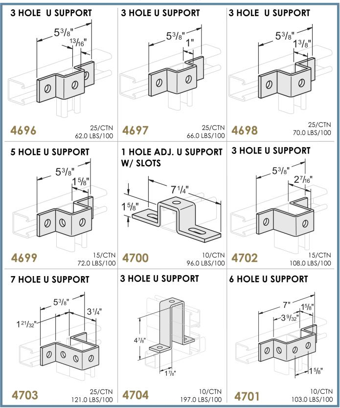
UNLESS SPECIFIED, MATERIAL IS 1-5/8" WIDE. HOLES ARE 9/16" DIAMETER, 13/16" CENTER TO EDGE, & SPACED 1-7/8" ON CENTER.
