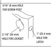
Drill 2-1/8" (54 mm) hole through door face as marked for lockset. (It is recommended that holes be drilled from both sides on wood doors to prevent splitting.) Drill 5/16" (8 mm) holes for screwposts. Drill 1" (25.4 mm) hole in center of door edge for latch.
