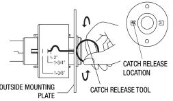
B. Install removable screw post into slots on outside mounting plate. Install rose liner and align rose liner arrow in the direction of the lock stile. Install outside rose and lever onto lock body assembly.
