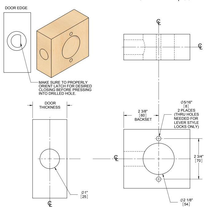
**NOTE:** INSERT LATCH INTO  $\phi$ 1"[25] HOLE USING FINGER PRESSURE. THEN WHILE HOLDING A PIECE OF WOOD OVER THE LATCH FACE, STRIKE WITH A MALLET UNTIL LATCH IS SITTING FLUSH WITH DOOR EDGE.
