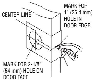
Measure center line of lock; height as desired from finished floor. Select 2-3/4" or optional 2-3/8" backset, fold and apply template to interior side of door and mark center of door as indicated on template. Mark center hole on door face through guide on template.
