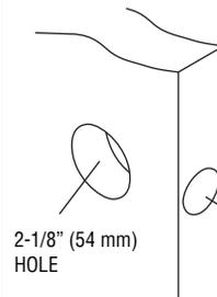
Drill 2-1/8" (54 mm) hole through door face as marked for lockset. (It is recommended that holes be drilled from both sides on wood doors to prevent splitting.) Drill 1" (25.4 mm) hole in center of door edge for latch.
