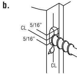
Drill (2) 1"(25.4 mm) holes 1-1/4" (31.7 mm) deep in door jamb, 5/16" (8 mm) above and 5/16" (8 mm) below horizontal center line.
