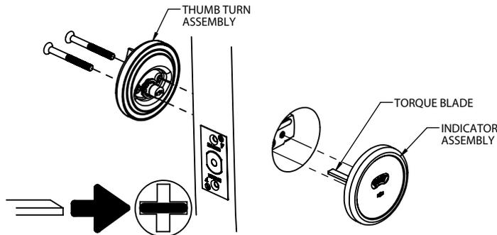
Insert torque blade horizontally into deadbolt latch. Crank until indicator assy is flush with the door face. Mate the thumbturn assembly with the torque blade on the indicator assembly. Insert the screws thru the holes of the thumbturn assembly and latch body. Tighten the screws to the threaded posts of the blank mounting plate. Tighten the assembly so the complete assembly is tight to the door.
