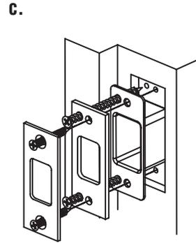
Match screw holes on strike with vertical centerlines on jamb. Mark outline of strike and chisel 1/4" (6.4mm) deep for flush fit of dust box, wood frame reinforcer, and strike. Place dust box and wood frame reinforcer into mortised area and tighten to the frame using 3" wood screws. Insert the strike and tighten to the frame with #8 screws.
