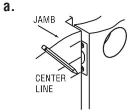
Close door. Locate strike in jamb and center line of strike. Open door and extend line to door stop. Measure half of door thickness plus 1/8" from door stop. Vertically mark centerline for strike.
