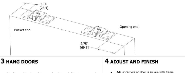
Open quick release latches on brackets and slide door onto carriers and close latches.
